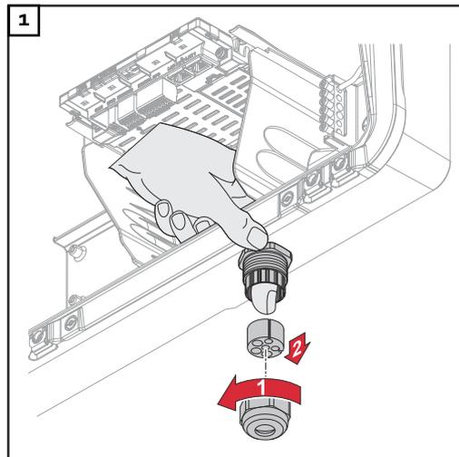
Undo the strain-relief device cap nut and push out the sealing ring and the blanking plug from the inside of the device.
