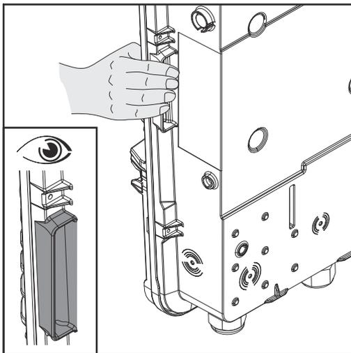
There are integrated grips on the side of the inverter which facilitate lifting/ attaching.
