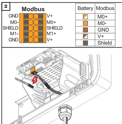
Insert the cable into the respective slot and check the cable is securely retained.
