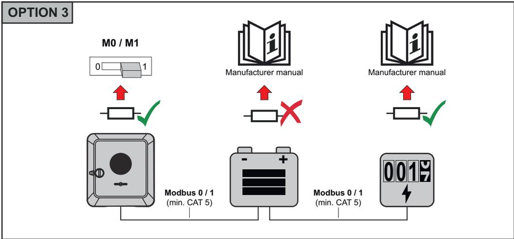
**Installing the WSD (wired shutdown)**
