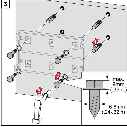
**Installing the mounting bracket on a mast or beam**
