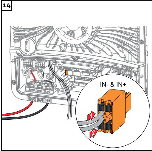
Connect the signal cable to the push-in WSD terminal on the IN- and IN+ slots, observing the labelling.
