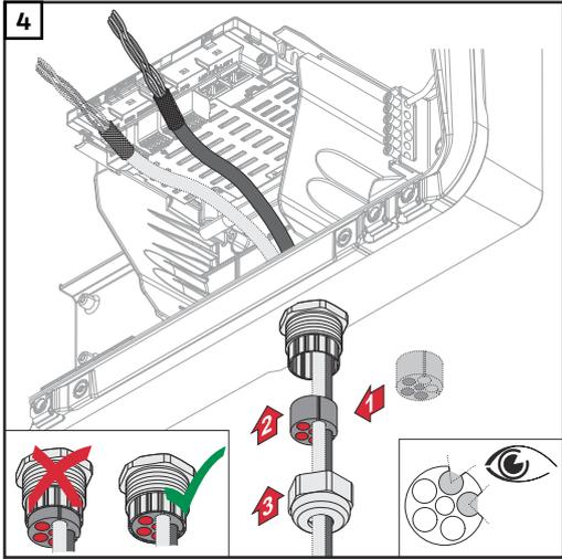
Insert the sealing ring between the cap nut and the housing opening. Press the data cables into the seal's cable guide. Then press in the seal until it reaches the underside of the strain-relief device.
