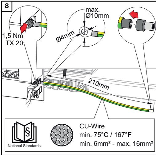
**IMPORTANT!** Depending on national standards and guidelines, a larger cross section of the ground conductor may be required.
