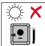
In order to minimise the heating up of the inverter, do not expose it to direct insolation. The inverter should be installed in a protected location, for example, below the PV modules or under an overhanging roof.
