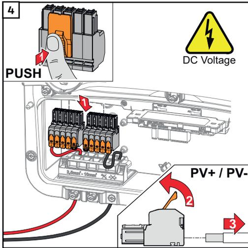
Remove the DC push-in terminals from the slots and disconnect them from the cables (only necessary if the installation already exists).
