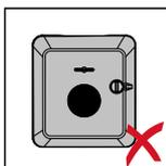
Do not install the inverter on a vertical wall or pillar with its connection sockets facing upwards.
