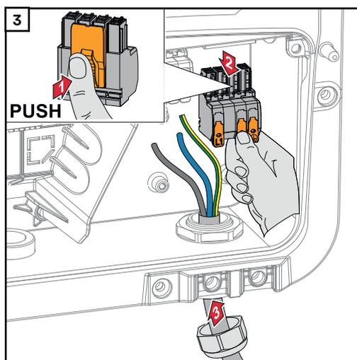
Guide the mains cable from below through the strain-relief device on the right side. Remove the AC terminal.
