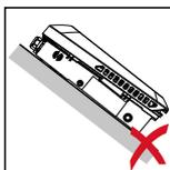
Do not install the inverter on a sloping surface with its connection sockets at the top.
