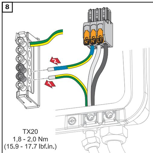
Fasten the ground conductor and PEN conductor to the ground electrode terminal using a screwdriver (TX20) and a torque of 1.8-2 Nm.
