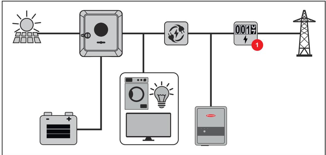
**Operating mode – Inverter with battery, further inverter and backup power function**
