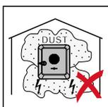
The inverter is essentially designed to be dustproof (IP 66). In areas of high dust accumulation, dust deposits may collect on the cooling surfaces, and thus impair the thermal performance. Regular cleaning is required in this case, see chapter **Operation in dusty environments** on page 151. We therefore recommend not installing the inverter in areas and environments with high dust accumulation.
