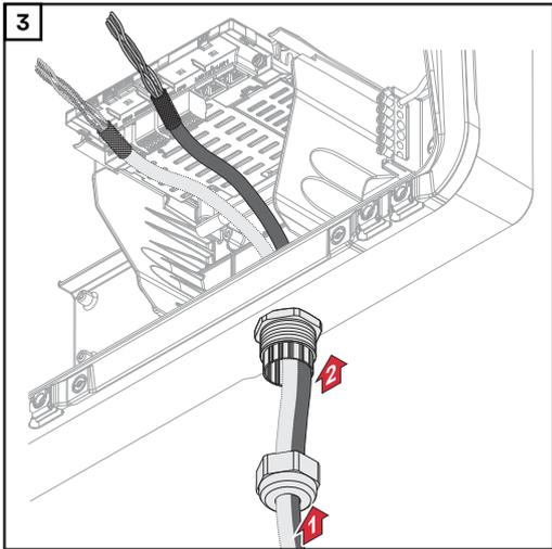
Guide the data cables first through the strain-relief device cap nut and then through the housing opening.
