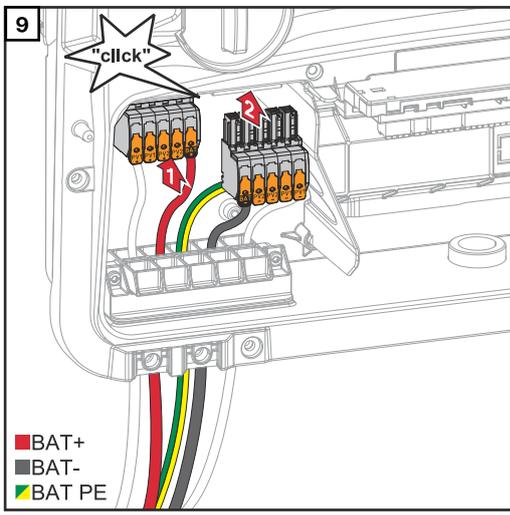
Insert the DC terminals into the respective slot until they engage.
