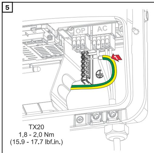
Fasten the battery ground conductor to the second input of the ground electrode terminal from above using a screwdriver (TX20) and a torque of 1.8-2 Nm.
