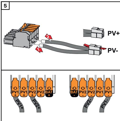
Connect the supplied PV+/PV- cables to the respective connections.
