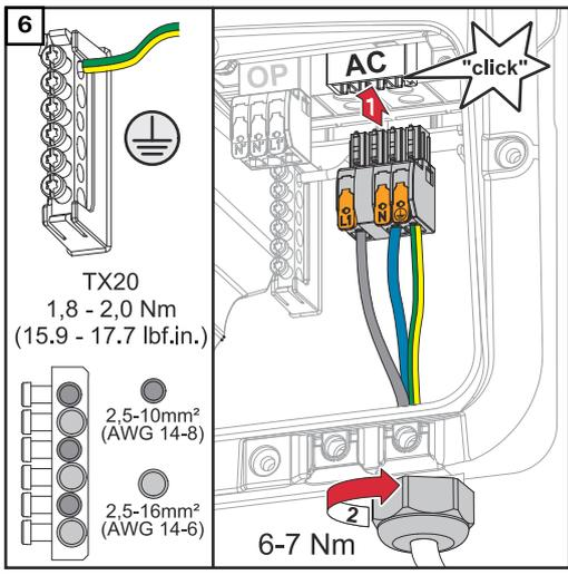
Insert the AC terminal into the AC slot until it engages. Fasten the cap nut of the strain-relief device with a torque of 6-7 Nm.
