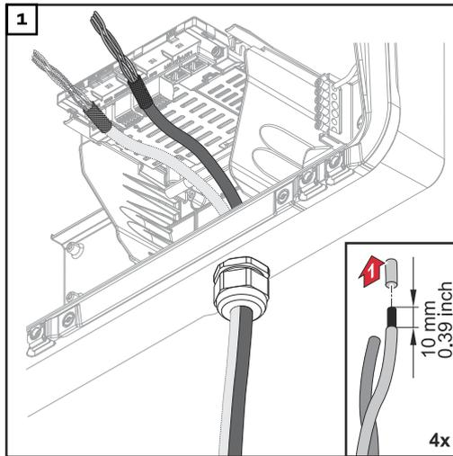
Strip 10 mm from the single conductors and mount the ferrules if necessary.
