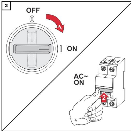
Set the DC disconnecter to the "On" switch position. Switch on the automatic circuit breaker.
