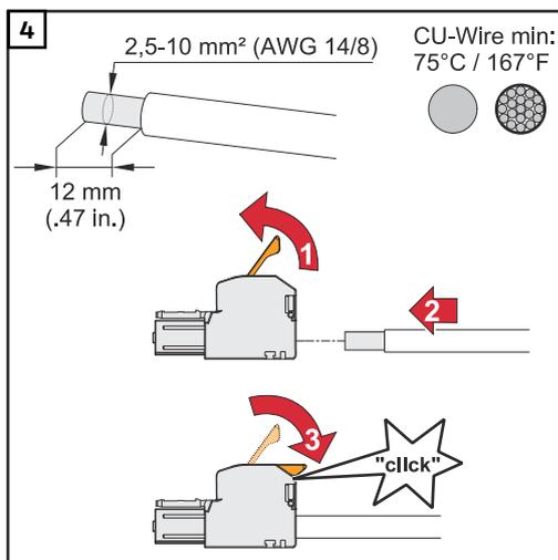
Strip the insulation of the single conductors by 12 mm. Select the cable cross section in accordance with the instructions in [Permitted cables](#) from page 61. Lift to open the terminal's operating lever and insert the stripped single conductor into the slot provided as far as it will go. Then close the terminal's operating lever until it engages.
