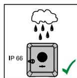
The inverter is suitable for outdoor installation.
