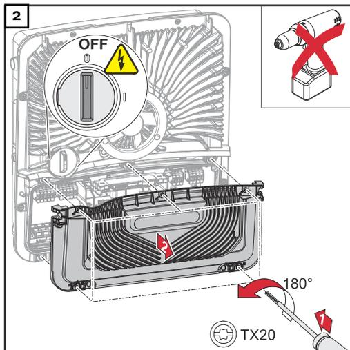
Make sure that the DC disconnecter is in the "Off" switch setting. Loosen the five screws of the connection area cover by rotating them 180° to the left using a screwdriver (TX20). Remove the connection area cover from the device.
