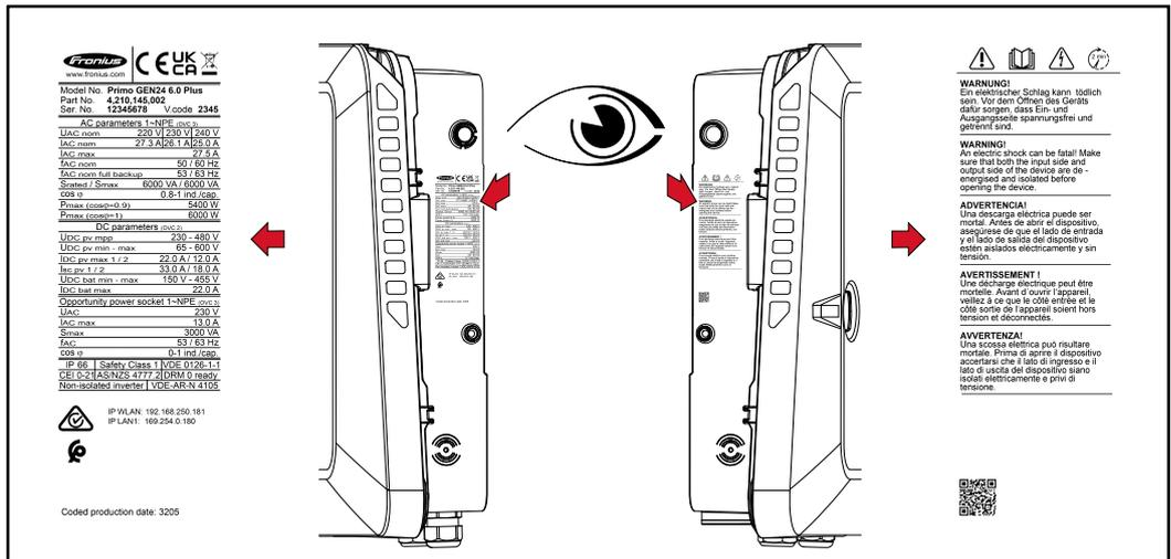
A 4-digit number (coded production date) is printed on the rating plate at the very bottom, from which the production date can be calculated. If you subtract the value 11 from the first two digits, you get the production year. The last two digits stand for the calendar week in which the device was produced.
