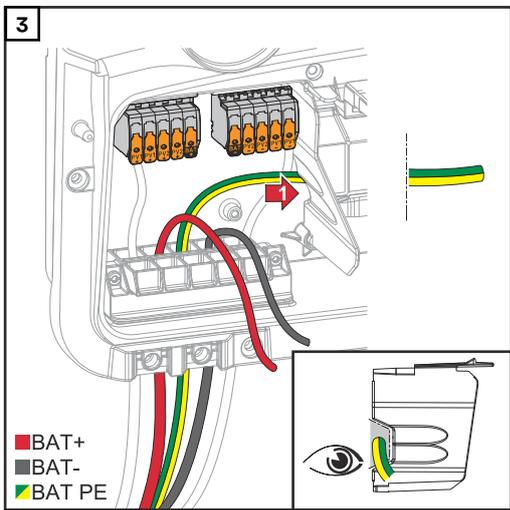
Route the battery ground conductor in the integrated cable duct of the connection area divider into the AC connection area.
