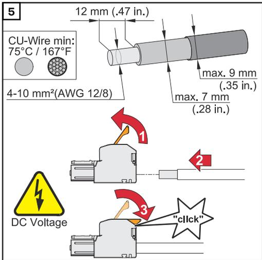
Select the cable cross section in accordance with the instructions in **Permitted cables** from page 61. Strip the insulation of the single conductors by 12 mm. Lift to open the terminal's operating lever and insert the stripped single conductor into the slot provided, in each case as far as it will go. Then close the operating lever until it engages.
