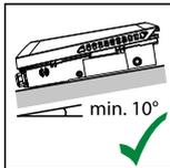
The inverter is suitable for installation on a sloping surface (min. slope to underside 10°).
