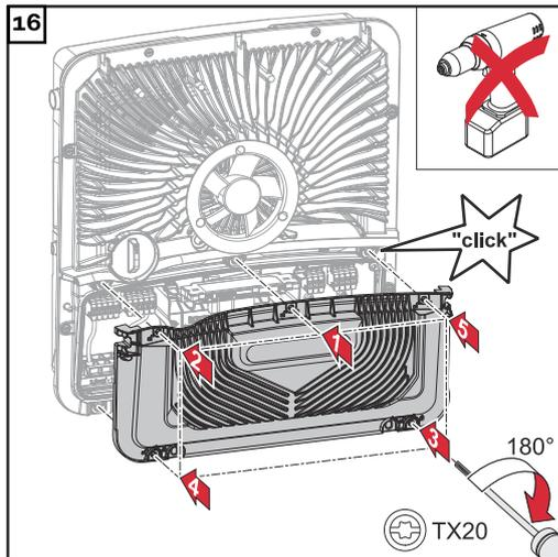
Place the cover on the connection area. Tighten the five screws by rotating them 180° to the right in the indicated order using a screwdriver (TX20).
