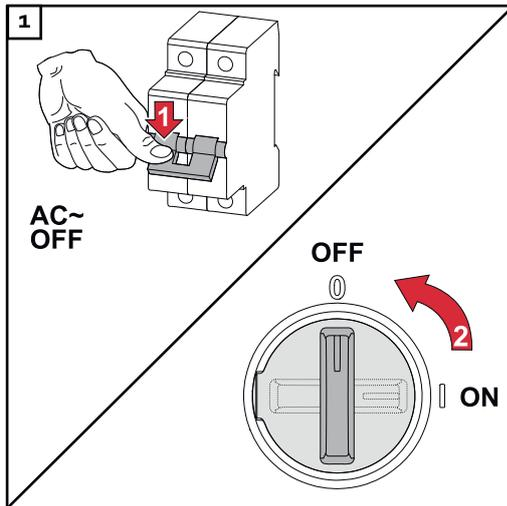
Switch off power to the inverter and wait for the specified time until the capacitors have discharged and the fan has shut down.
