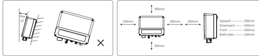
To allow for a dissipation of the heat and in order to facilitate dismantling, the space around the inverter should allow for some clear spaces. The spacing around inverter should meet the requirements as illustrated in below figures for the sake of heat dissipation and demounting.
