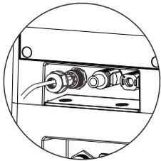
3. Plug the other end of the CAN communication cable to the CAN connector on BMS. Tighten the screw cap at the end of the cable.
