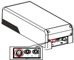
2. There's a protect cap for the CAN connector on BMS, unscrew the cap.
