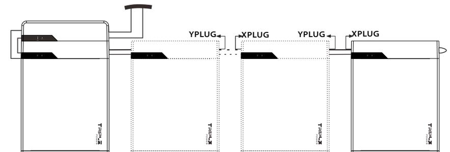
2. After all the battery modules were correctly connected, plug the short-circuit plug (F) at YPLUG (V) of last battery module to make a complete circuit.
