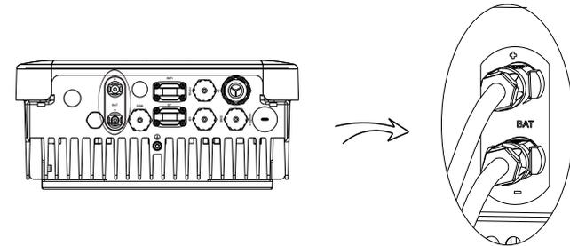
2. Connect the negative cable (-) (B) to the port on the right and the positive cable (+) (A) to the one on the left shown as in the figure.
