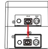
2. Please make sure that both ends of the power cable are connected to the correct connector, which are on the left side of BMS and battery module that shown in the figure.
