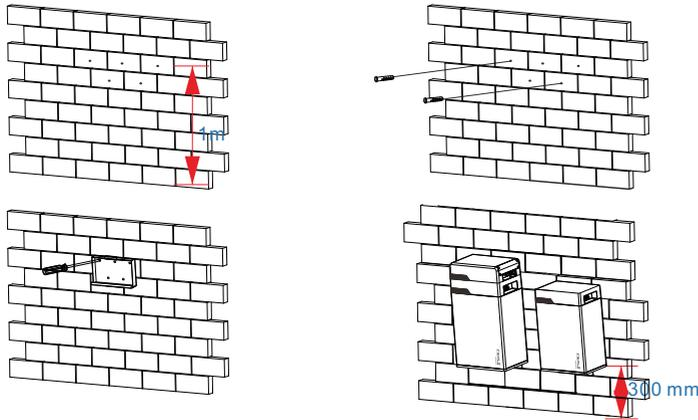
The following figure is the back view of wall mounting.
