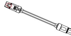
1. Plug either end of the 120mm power cable into the XPLUG port on BMS, and the other end into the XPLUG port on battery module. When the metal sheet which is marked in red is totally inserted and a click sound is heard, that means the power cable is properly connected.
