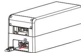
3. Once finished, please connect the short-circuit plug to the YPLUG port on battery module(V') to complete the internal circuit.
