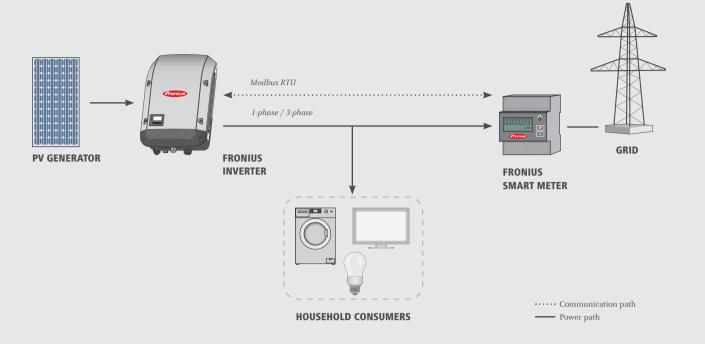
/ The Fronius Smart Meter is compatible with all inverters with an RS485 interface (Modbus RTU). The Fronius Smart Meter works in conjunction with the Fronius Datamanager 2.0 for the Fronius IG Plus inverters. The Fronius Smart Meter can be retrofitted at any time together with the Fronius Datamanager 2.0 in inverters that have already been installed.
