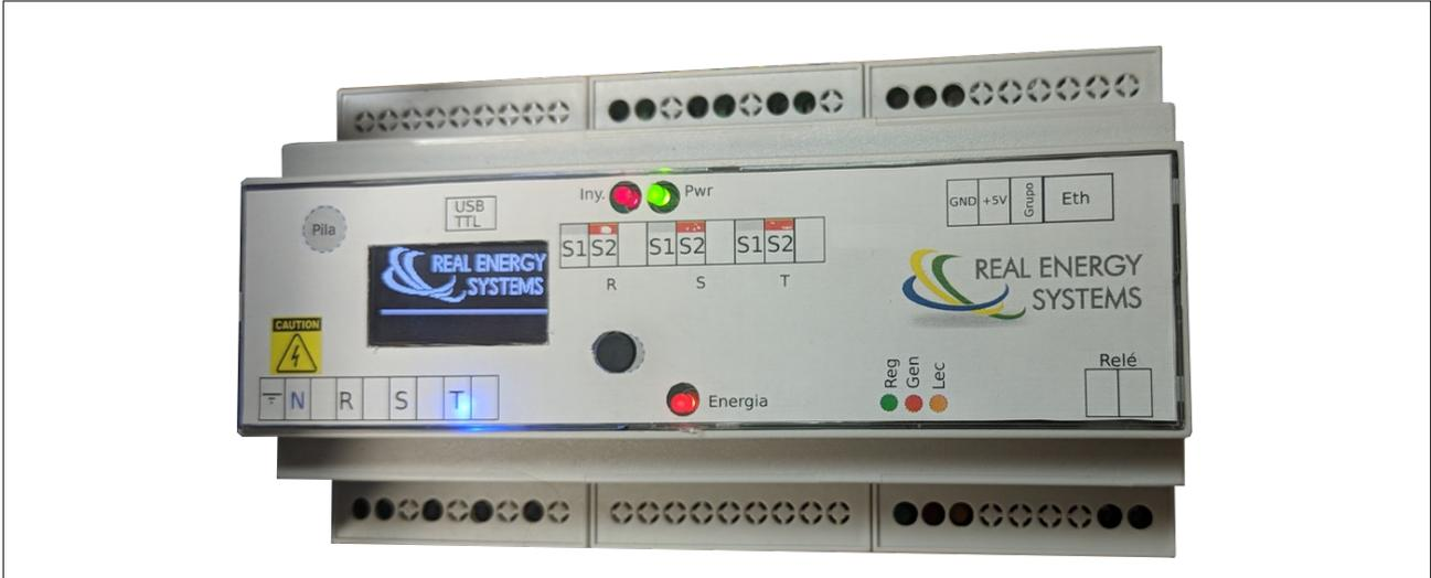
Figure 1 PRISMA 310A - allows power regulation
