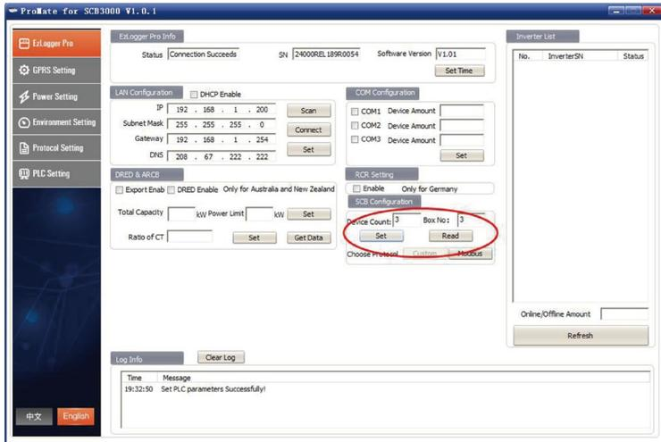
Note: The Device Count and Box No are required, the devices will not function properly if either field is not filled in.
