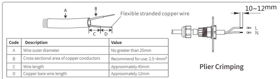
Note: Before connecting the AC power line, make sure that the switch upstream of SCB3000 is open
