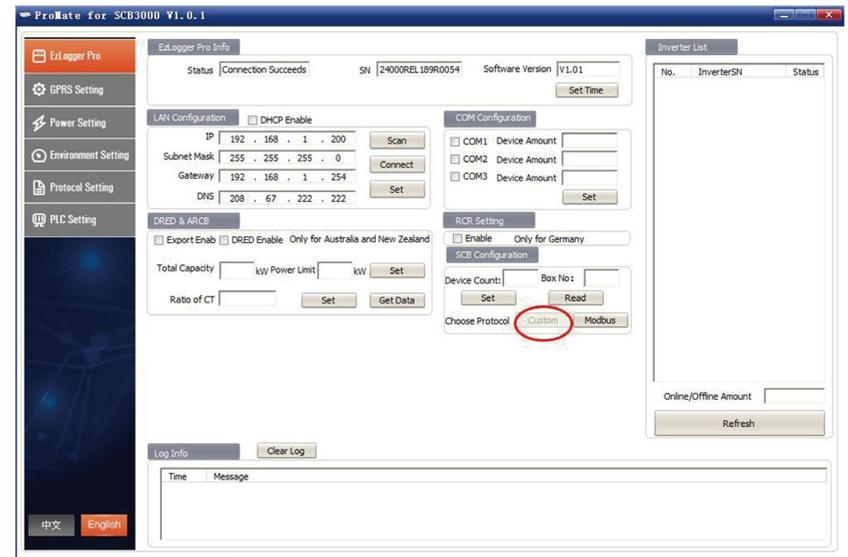
Note: Select the GOODWE custom protocol first to configure the BOX No and inverter address, then switch to the Modbus protocol for communications after all parameters have been configured.
