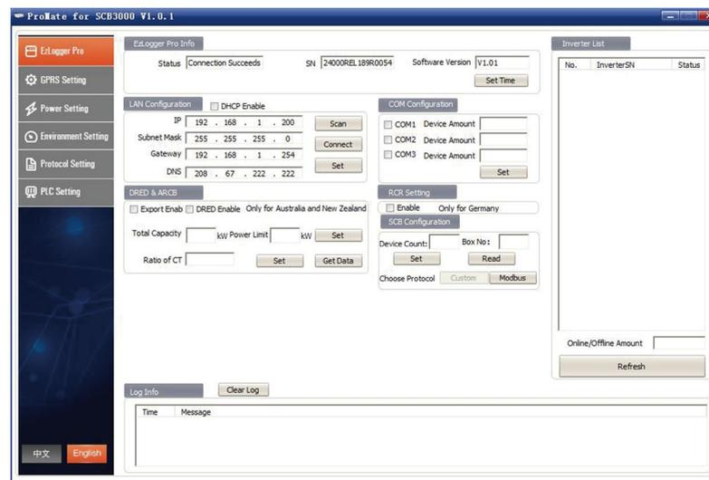
Note: If the SCB3000 is set to static IP mode, you need to switch to dynamic IP mode before you can configure it using dynamic IP connection. Press and hold the "RELOAD" button for about 4 seconds, this will make the LED signal indicators flash from right to left, indicating a completed reset and restart, after which the SCB3000 will be switched to static IP mode.
