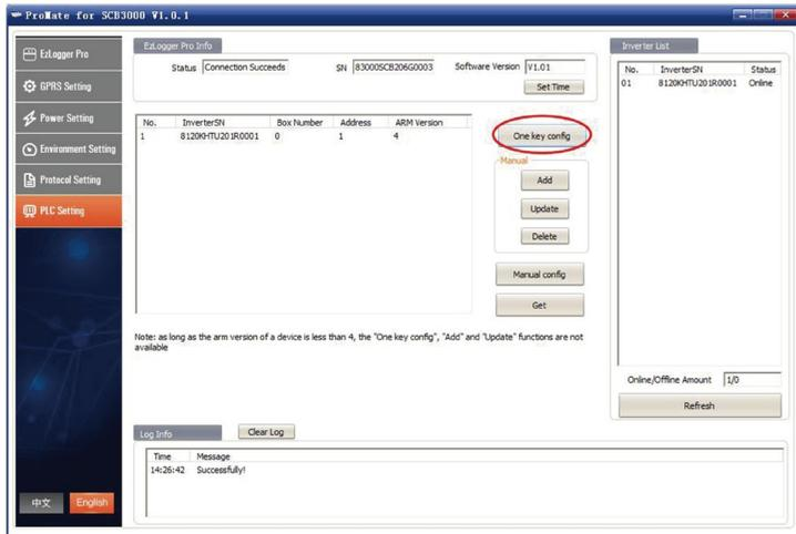
As shown below: If you need to modify the Modbus address after adding it, you can select the inverter serial number that needs to be modified, click the "Update" button, enter the parameters to be modified in the popup dialog box, click "OK" and then click "Manual config".
