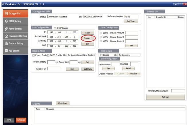
Note: If there is only one Box-type substation on the customer site, and the data is uploaded to GOODWE servers, there is no need to configure the box number and address through ProMate, simply connect ProMate, click to get the inverter list to see if the inverter is all online. If there are multiple box Box-type substations onsite, refer to 5.2.2 for setup.
