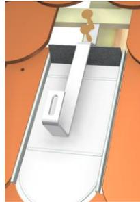
Insert roof hook with the bracket positioned in the trough of the roof tile. Mark the top tile and, if necessary, the bottom tile at the roof hook exit point. If the distance to the tile cannot be maintained, use additional support plates (optional component). For plain tile covering follow the instructions in the clamping system mounting versions (MV 2).
