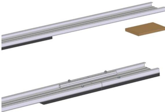
If the base trough 150-30 w/cross drainage has to be cut to size on site and then starts/ends without a PE-pad, then a PE pad must also be applied on.
