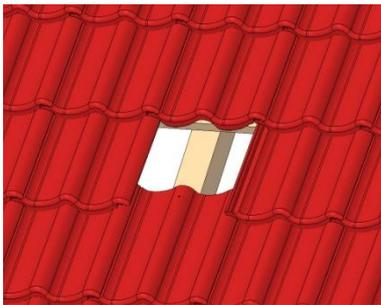
Expose the rafters by removing the tiles.
