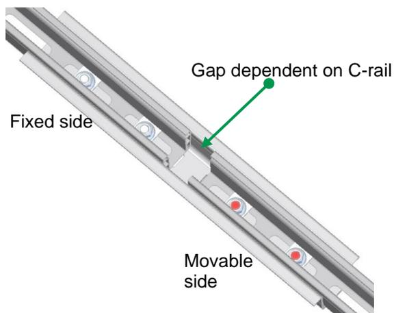
Place rail ends onto the gap, apply the rail connector and connect it to the rail at the fixed and movable sides using the mounting screws. Tighten the screws firmly on the fixed side. The screws on the movable side are coated in red and must be released again after tightening (approx. ½ turn). Maximum rail length with expansion joint 40 m, then plan proper rail disconnection.
