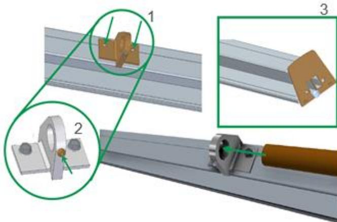
The mounting brackets snowguard IR have to be fixed on the insertion rail Plus with two drilling screws (1). Position the round pipes centrally and fix them with the grub screw (2).
