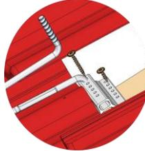
Attach the roof hooks to the rafter with wood screws (MV 1.4). The screw length depends on the roof design and is determined by the calculation software. If the counter battens were not taken into account in the design software or mounting is on a rafter insulation, the base profile of the roof hook must be padded on both sides of the counter batten for at least the width of the rafter.
