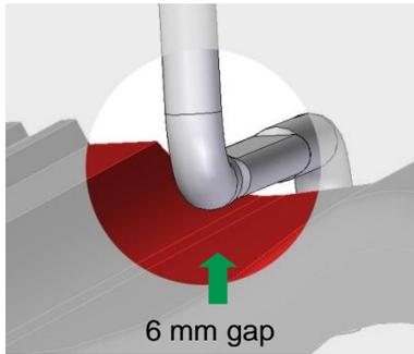
Height adjustment of the roof hooks through the thread in the base profile. The distance between the bottom tile and bracket must be 6 mm after attachment.
