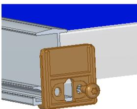
Fit an edge stop at the end of a module row at each insertion rail with a metal screw in the screw channel.
