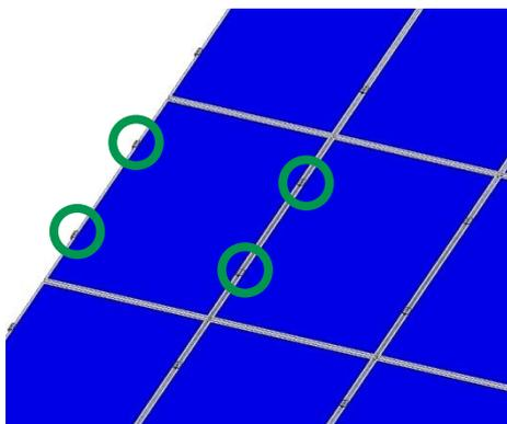
The modules must then be attached to the rails using end clamps and middle clamps.
