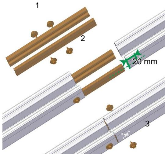
Push the rail connector set (1) half way into one of the rails to be connected (2) and secure it there with a drilling screw each on both sides approx. 20 mm from the rail end. Next push the other rail completely onto the rail connector set until both rail ends make contact (3) and screw it tight as described above. Maximum uninterrupted rail length 13 m, then install expansion joint.
