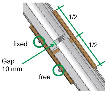
Centre the rail connector over the fitted rail and tighten the first threaded pin. Insert the rail to be connected into the connector, gap between the rails 10 mm, tighten the second threaded pin without play.
