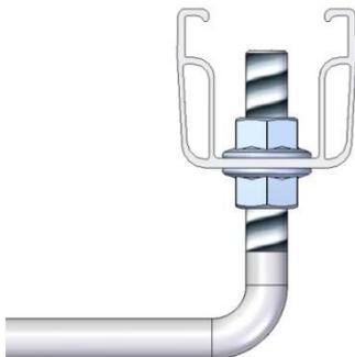
Place the C-rail onto the lower self-locking nut, align the rail and tighten it with the top self-locking nut. The roof hook can also be connected to the rail connector in the joint area. For mounting in the cross rail arrangement (insertion/clamping system) the top rail is attached using the cross rail connector or Cross rail connector set C IR M8 (MV 2).
