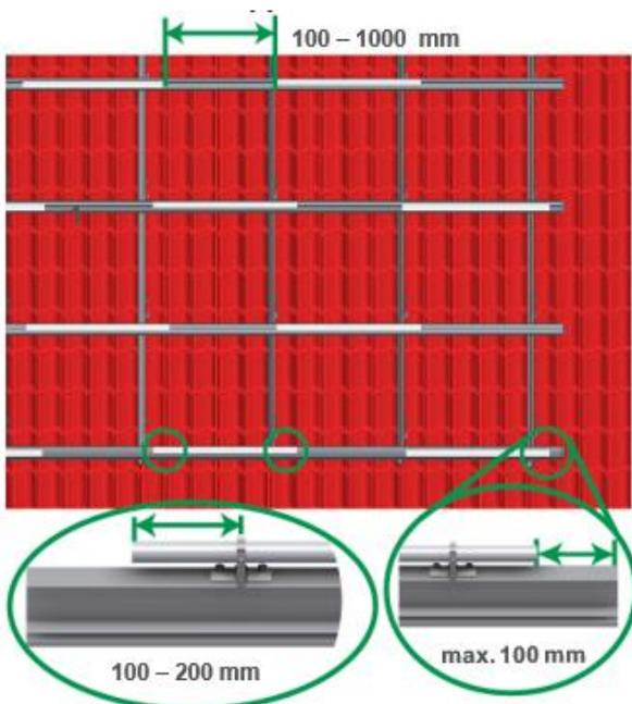
Distance between Aluminium round pipes at the end of the insertion rail in the corner area of the system max. 100 mm.
