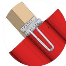
Insert roof hook with the bracket positioned in the trough of the roof tile. The position of the roof hook on the rafter must be defined taking into account the static specifications (MV 1.4). Mark the top tile and, if necessary, the bottom tile at the roof hook exit point. For plain tile covering proceed according to MV 1.2 + 1.3.
