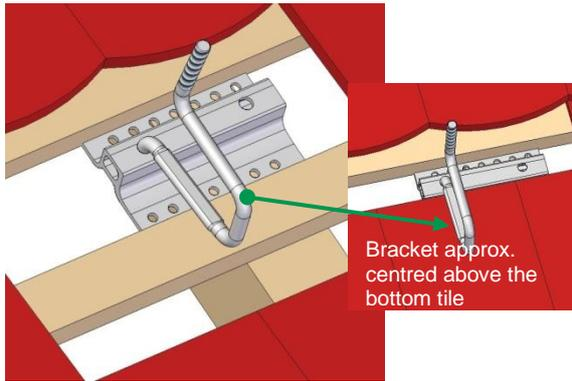
Install the roof hook with the long side of the base profile facing down. Position the bracket whilst maintaining the lateral overhang (MV 1.4) approx. centred above the tile below.
