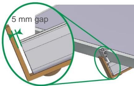
Screw the slip guard to the rail end with approx. 5 mm gap using mounting screw and self-locking nut.
