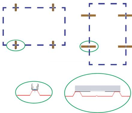
Mark the mounting position of the short profiles on the trapezoidal metal raised beads dependent on the module orientation – portrait or landscape, right-angled or on the raised bead – and the clamping areas specified by the module manufacturer. A gap of min. 10 mm must be maintained between the modules at the short frame side.
