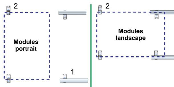
The short profiles with a length of 125 mm are to be placed on the inner side (1) of the top and bottom insertion rail and alternately on the top and bottom (2) of the middle insertion rails in accordance with the static calculation on the high beads and tightened with the required number of fasteners.
