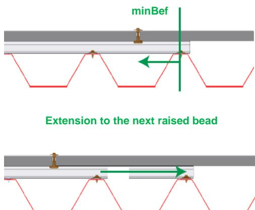
The distance (minBef.) between middle clamp and the next fastener in accordance with the static calculation must not be fallen below, if not observed, an extension to the next raised bead is necessary – this results in the min or max rail length.
