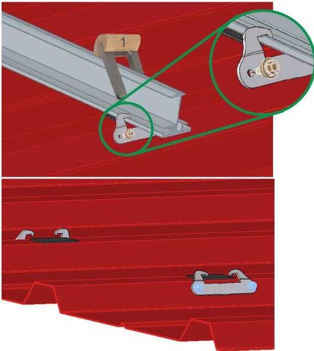
Position the trapezoidal sheet bracket with the aid of the mounting tool (1) on the insertion rail in the inclination of the raised bead with downward pressure. Screw the trapezoidal sheet bracket with two thin sheet metal screws into the side of the raised bead without predrilling.
