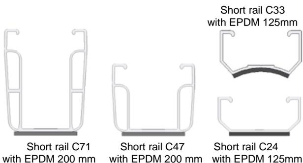
To improve ventilation behind the modules the modules can be mounted using the short rail C47 or C71, the mounting steps must be carried out as described in chapter 5.1.
