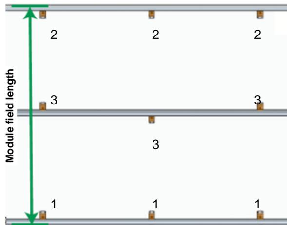
For the top and bottom insertion rail of the module field the Cross rail connector set C IR M8 is fitted on the inside in each case (1, 2), at the centre insertion rails the Cross rail connector set C IR M8 must be fitted alternating at the top and the bottom at the mounting flange (3).
