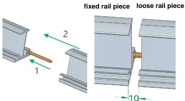
Push the connector into the secured rail piece up to half way into the screw channel, then push the loose rail piece with the screw channel onto the connector with a 10 mm gap between the rail ends, then attach the second rail piece.
