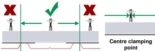
Position the end clamp or middle clamps in accordance with the adjacent figure.
