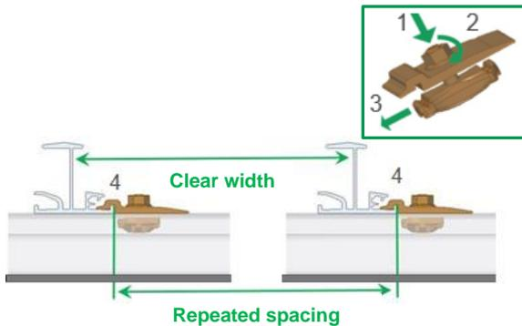
Insert the Cross rail connector set C IR from the top into the rail groove (1), rotate the nut by 90° (2) and push the component against the insertion rail (3) until Cross rail connector set C IR engages with the mounting flange (4).
