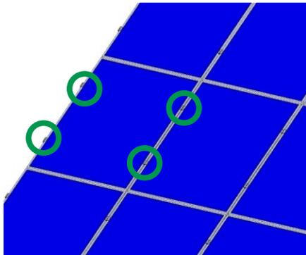
The modules must then be attached to the rails using end clamps and middle clamps – this applies analogously also to mounting the modules in landscape.
