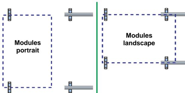
To improve ventilation behind the modules the modules can be mounted on short profiles.
