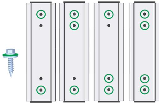
The static calculation in the system planning defines the number of fasteners required for mounting modules in landscape. For mounting modules in landscape the number of fasteners calculated with the design software is distributed on the raised bead as shown in the figure.
