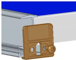
Fit an edge stop set IR at the end of a module row at each insertion rail with a metal screw in the screw channel.
