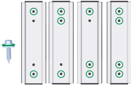
The number of fasteners is based on the static calculation with the fasteners shown.
