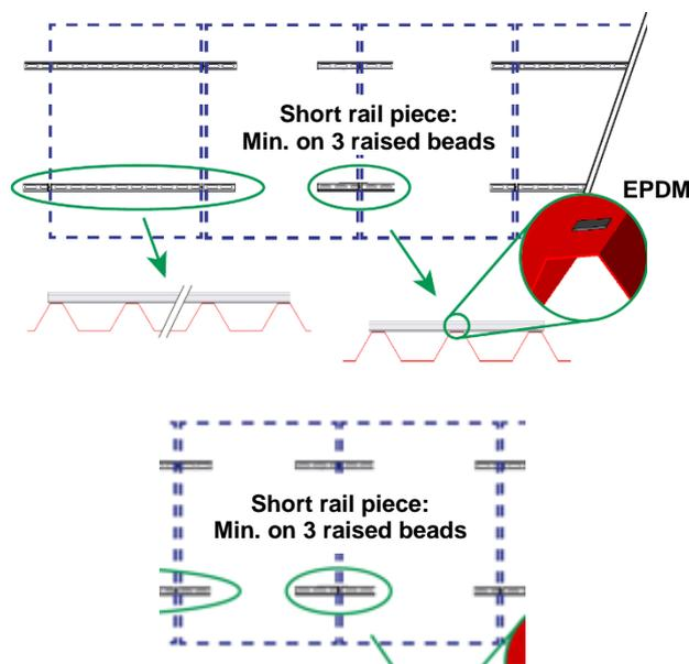
Mark the mounting axes of the rail pieces on the trapezoidal metal raised beads dependent on the clamping areas specified by the module manufacturer. Mark the position of the module clamps on these axes. Determine the length of the rail pieces from the Solar-Planit calculation dependent on the clamping position (taking into account MV 3.2 and 3.3) Glue EPDM sealing strips to the raised beads in the area of the rail pieces, fix the rail pieces to each raised bead across the rail piece length.
