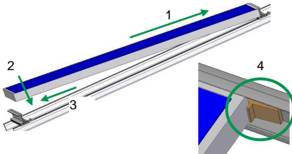
Place the module onto the top insertion rail and push it up (1). Then lower the module onto the bottom insertion rail (2) and push it down against the insertion rail (3). Mount the next modules following the same principle, the gap between the modules must be min. 3 mm.
