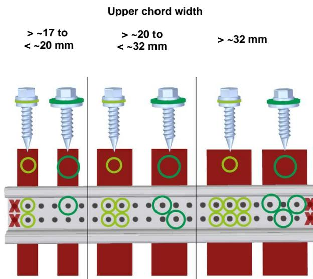
The static calculation in the system planning defines the number of fasteners required for mounting modules in portrait.
