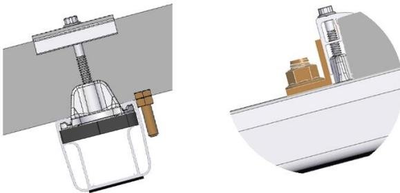
Prior to mounting modules in portrait, the module slip guards must be fitted to the frame holes above the bottom rail position (MV 3). For mounting modules in landscape module slip guard sets must be inserted at the lowest module row.
