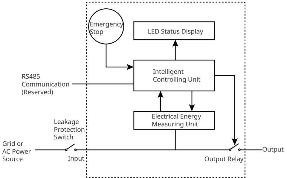
(Reserved) It is able to communicate with the inverters or smart meter via the RS485 communication port.
