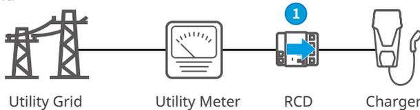
Turn on the RCD between the charger and the grid.
