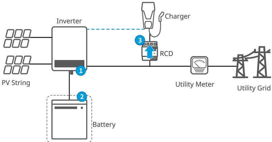
**Step 1** Turn on the AC and DC switches on the inverter side.
