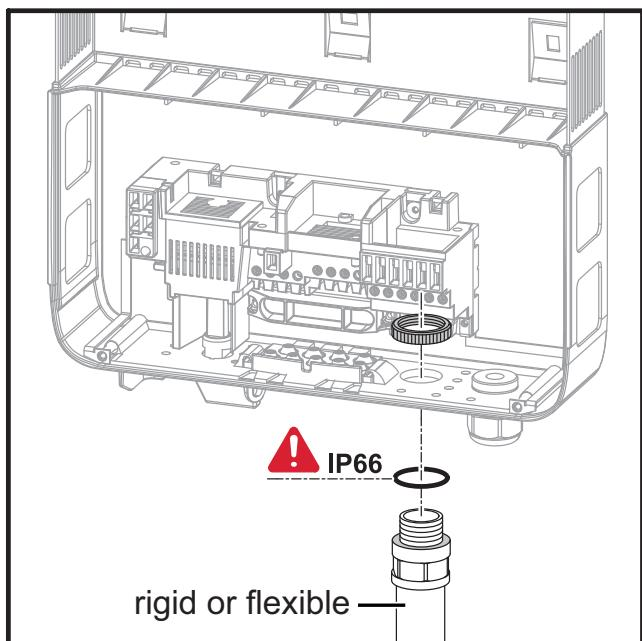
Ensure that the cable protection hoses are tightly sealed.
