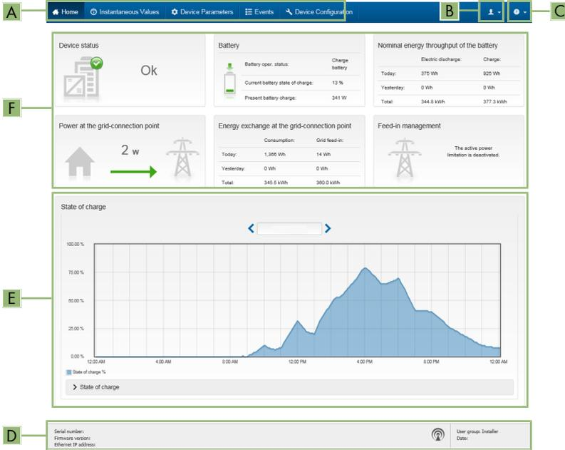
Figure 26: Design of the user interface's home page (example)
