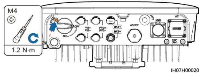
**Step 5** Install the SUN2000 on the mounting bracket.
