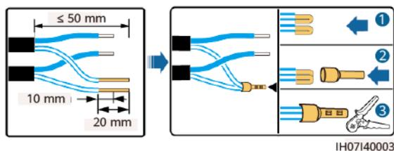
**Figure 5-24** Crimping three signal cables
