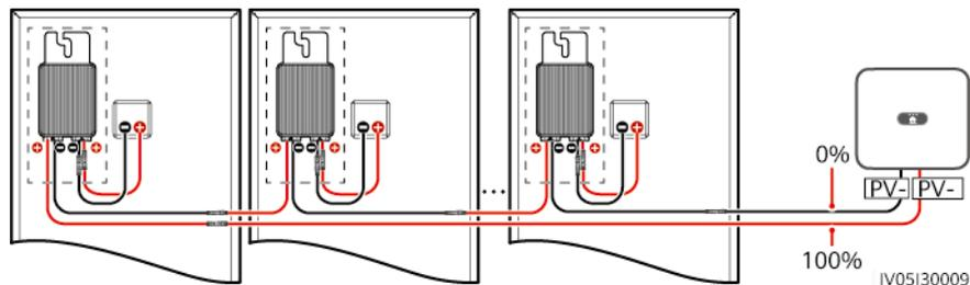
**Step 4** Set the DC switch to OFF and check whether the connector or DC cable between the possible faulty PV modules and the corresponding optimizers, or those between the adjacent PV modules and the corresponding optimizers are damaged.
