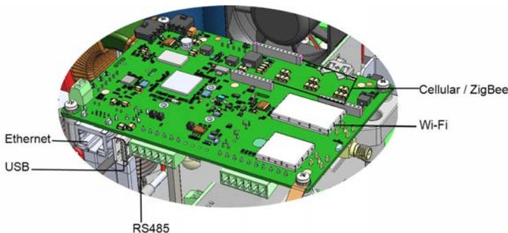
Figure 16: Internal connectors
