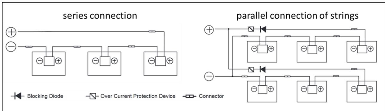
Suitable overcurrent protection measures (e.g. string cut-out) are required for the parallel connection of the modules. It must be ensured that the specified capacity regarding the return current IR of the datasheet will not be exceeded. If there are more than two parallel strings, string fuses and string diodes must be used.
