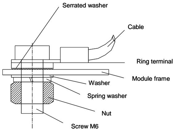
The modules are to be grounded according to the country-specific requirements and laws. If a lightning protection system is already present or intended to be installed on the building, the PV system is to be integrated into the protection concept against direct lightning strike. If a transformerless inverter is used, equipotential bonding may be prescribed in accordance with the inverter manufacturer's specifications. Country-specific laws must be observed.
