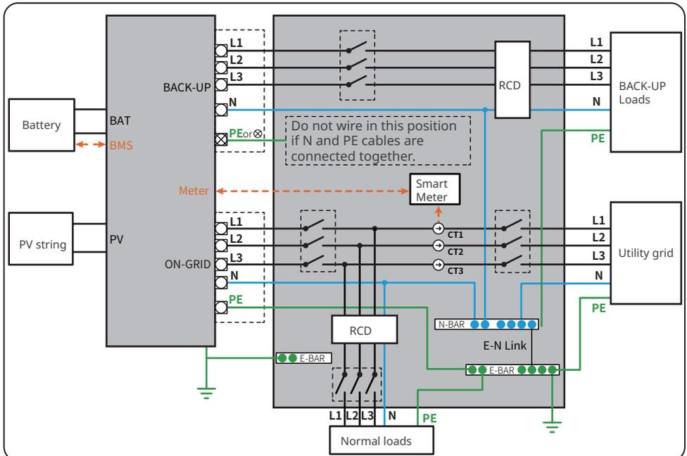
**N and PE cables are separately wired in the Main Panel.**
