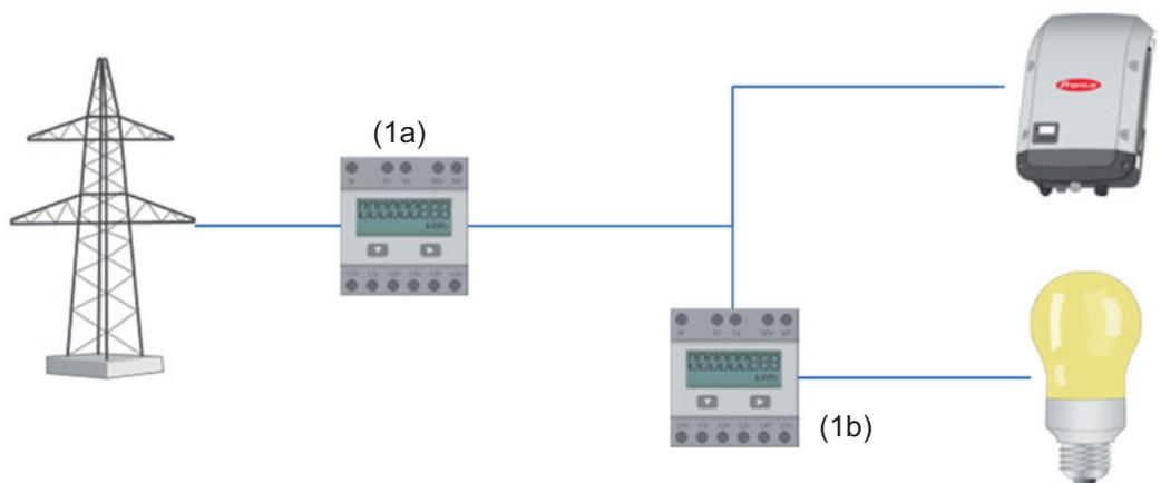
A meter for recording self-consumption per S0 can be connected directly to the inverter.
