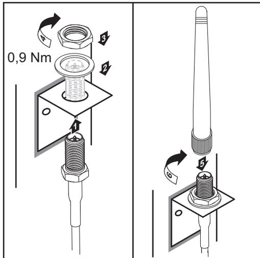
**7** Run the antenna cable through the drill hole on the mounting bracket
