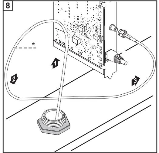
\*Bending radius of the antenna cable: at least 25.4 mm/1 in.
