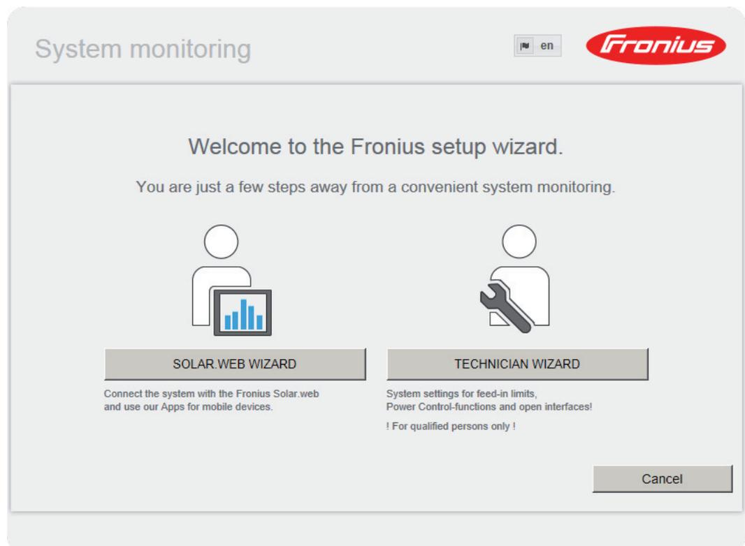
The Technician Wizard is designed for the installer and includes standard-specific settings. If the Technician Wizard is run, it is essential to note down the assigned service password. This service password is required to configure the UC Editor and Meter menu items. If the Technician Wizard is not run, no specifications for power reduction are set.
