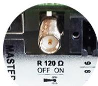
**IMPORTANT!** The termination resistance must be active for the first and last device in an RS485 bus.
