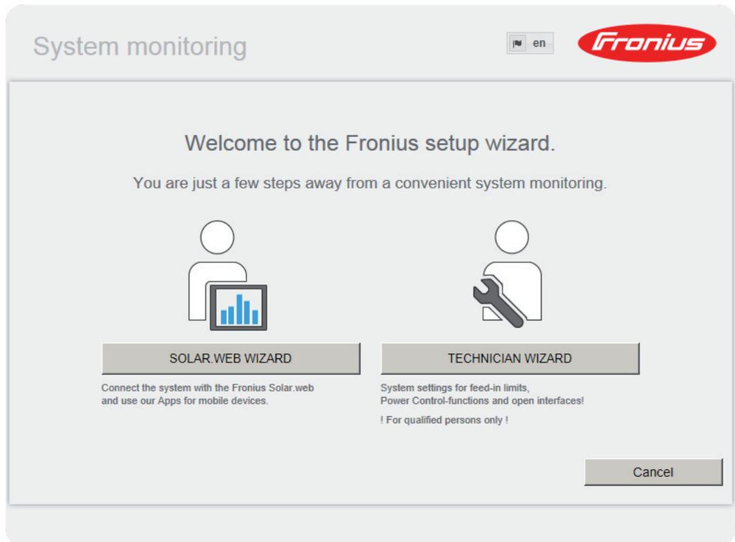
The Technician Wizard is designed for the installer and includes standard-specific settings. **Running the Technician Wizard is optional.**
