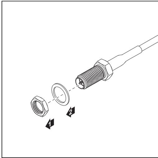
**6** Remove the hex nut and washer from the outside thread of the antenna cable
