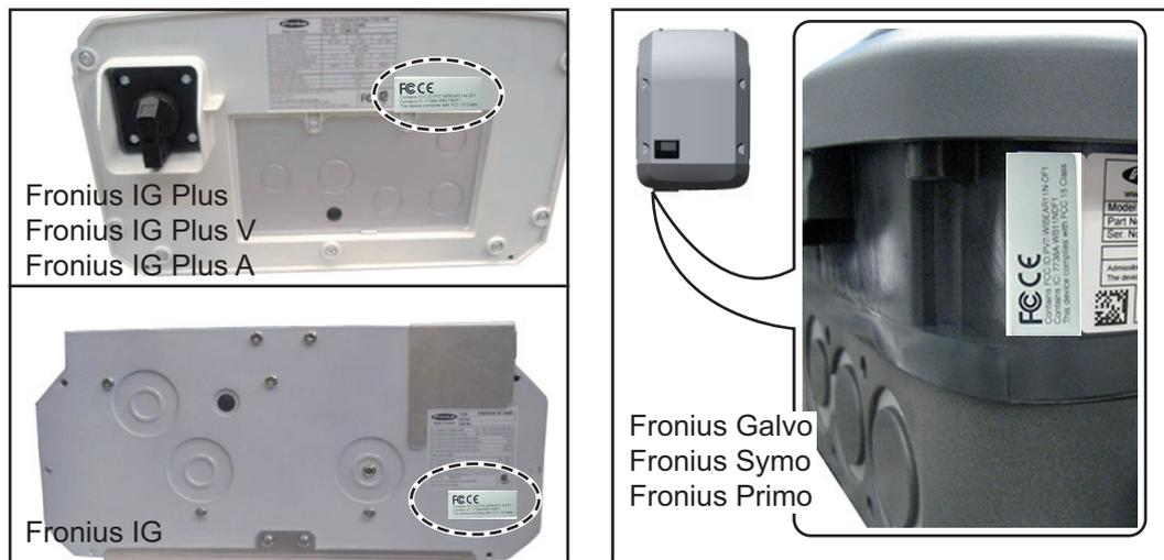
For Fronius Galvo, Fronius Symo, and Fronius Primo inverters, the sticker label information is located on the rating plate.
