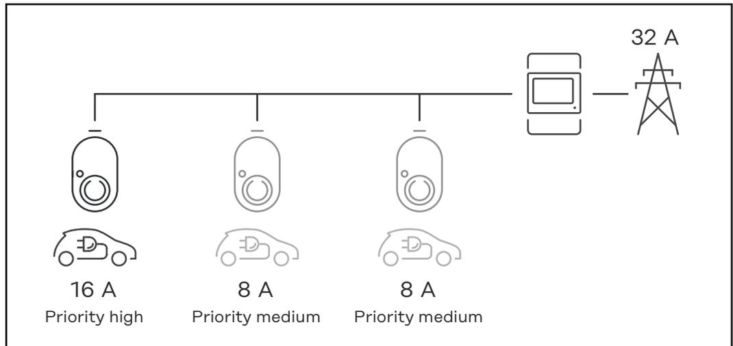
Distribution of the charging current with three Wattpilots with different priorities (one with high priority, two with medium priority).
