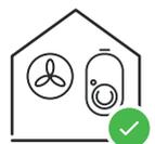
The Wattpilot is suitable for operation in a well-ventilated indoor area.
