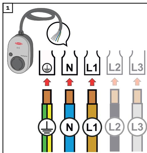
Have the 5-pin mains cable connected by an authorised electrician in accordance with national standards and safety rules. Depending on the available mains supply type, opt for a 1- or 3-phase connection.
