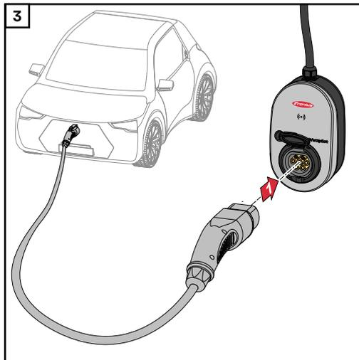
Connect a Type 2 to Type 2/Type 1 charging cable to the Wattpilot and the car.
