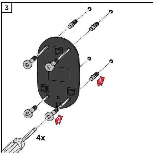
Place dowels in the holes and fasten the mounting bracket with screws.
