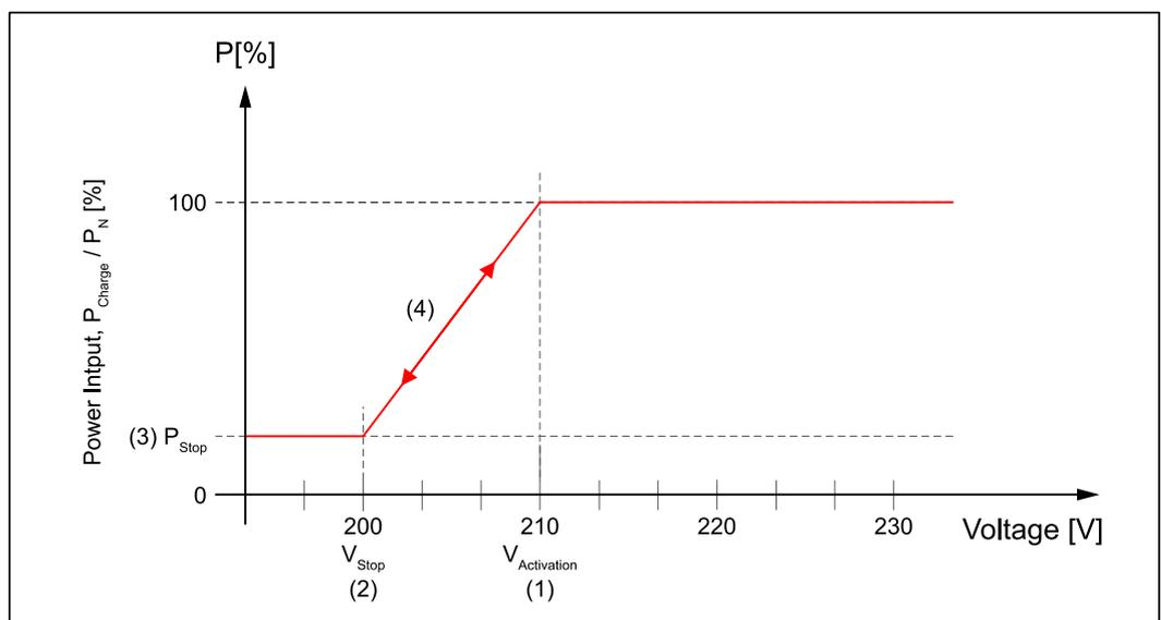
Charge power limitation when "Activation Threshold Undervoltage" is exceeded.
