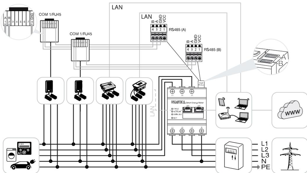
In a multiple-inverter connection, up to 10 KOSTAL inverters can be used in the same house grid.
