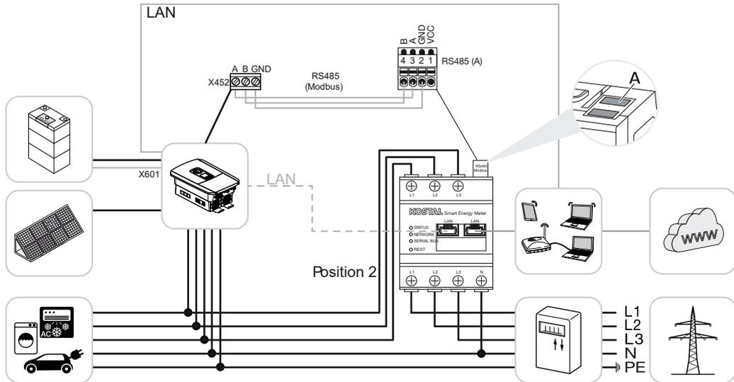
Install the KOSTAL Smart Energy Meter in the house grid as shown.
