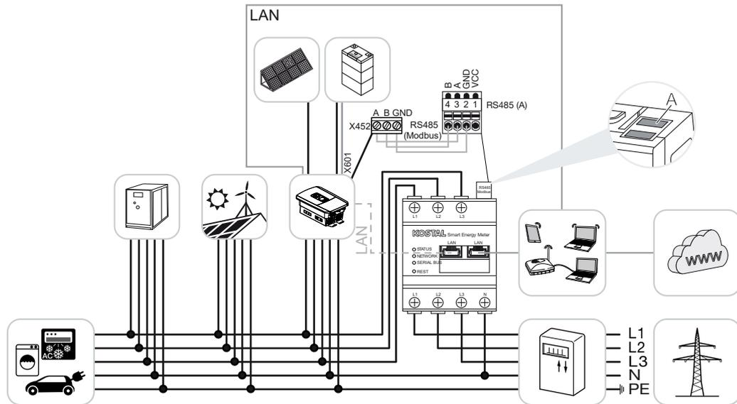
Install KOSTAL Smart Energy Meter as shown at the grid connection point (position 2) in the house grid.
