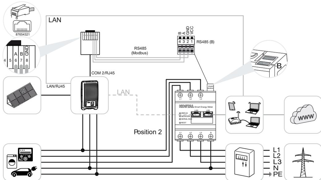
Install the KOSTAL Smart Energy Meter in the house grid as shown.
