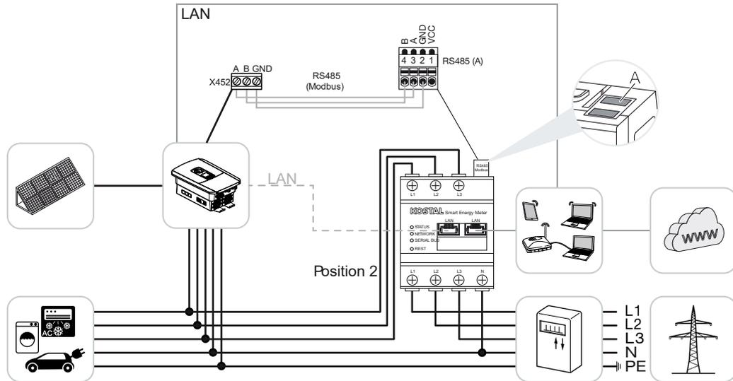
Install KOSTAL Smart Energy Meter as shown for home consumption (position 1) or at the grid connection point (position 2) in the house grid.
