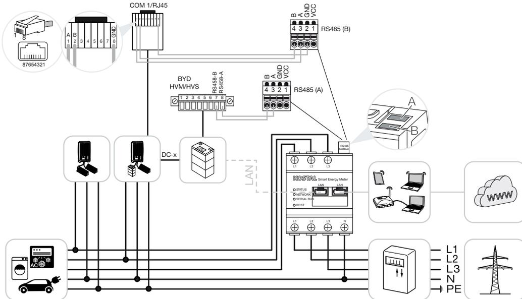
Install the KOSTAL Smart Energy Meter at the grid connection point in the house grid as shown.
