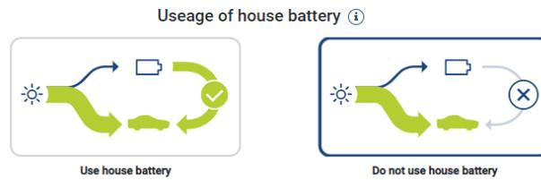
If there is a battery in the house network, this will also be used to charge the electric vehicle as standard.
