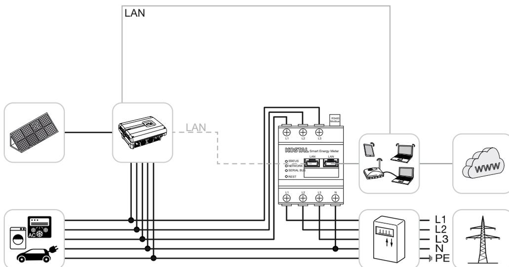
Install KOSTAL Smart Energy Meter at the grid connection point in the house grid as shown.
