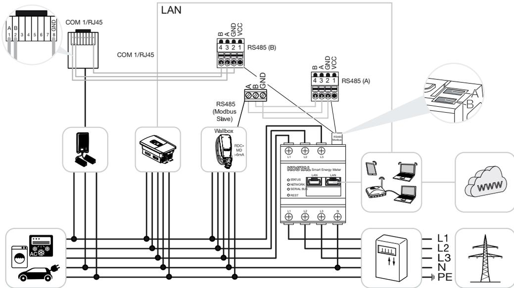
Only one KOSTAL Smart Energy Meter is required to monitor power and limit feed-in at the grid connection point. This is installed at the grid connection point in the house grid as shown in the illustrations.
