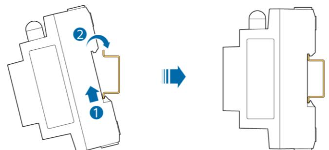
**EN** Install the EMMA on the DIN 35 mm standard guide rail of the AC power distribution box in which a surge protective device must be configured.
