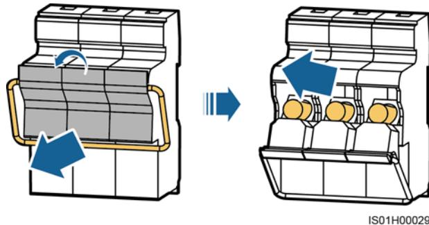
**Step 2** Install a new fuse and close the knife fuse switch box.
