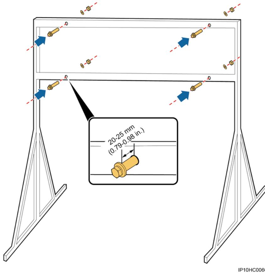
**Step 4** Assign two persons to lift the cabinet and mount it on the bolts, and assign another person to assist.
