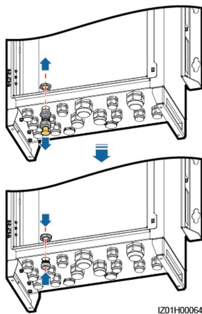
**Step 3** Route the cable through the tube conduit and then the fitting, and connect the cable.
