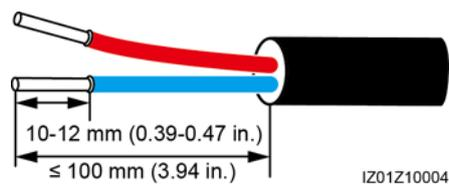
**Step 2** Connect the cable to the 24V OUT+ and 24V OUT- ports on the power module.
