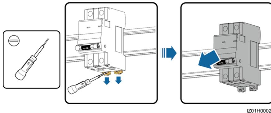
**Step 3** Install a new single-phase input switch.
