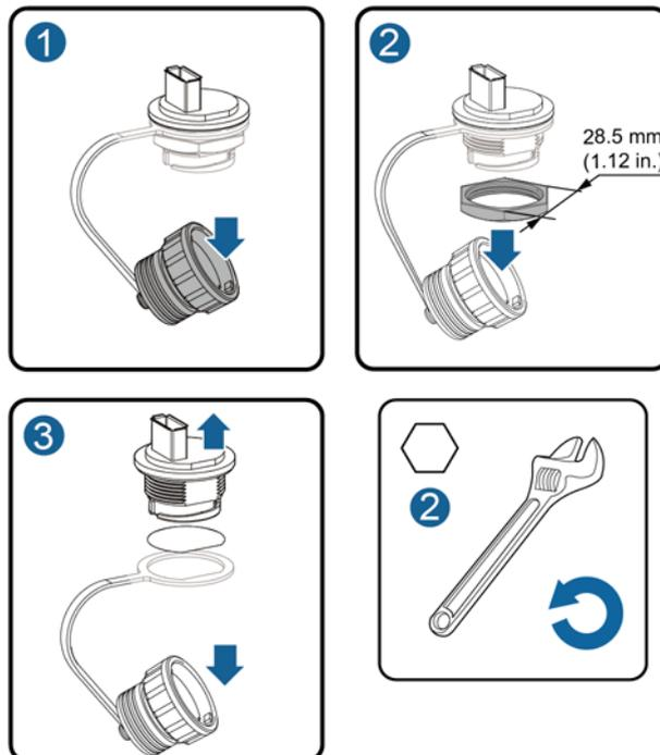
**Step 3** Ensure that the rubber ring is on the inner side of the cabinet when installing a new USB port.
