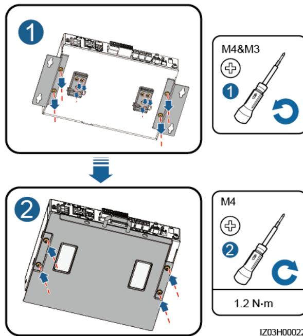
**Step 4** Install the new SmartLogger in the cabinet.
