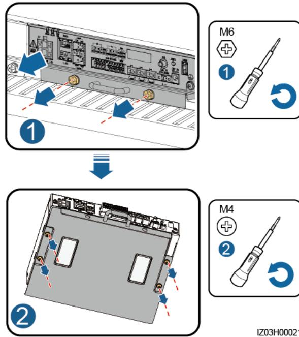
**Step 3** Remove the mounting ears and guide rail–mounting kit from a new SmartLogger, and install the cabinet-mounting kit.
