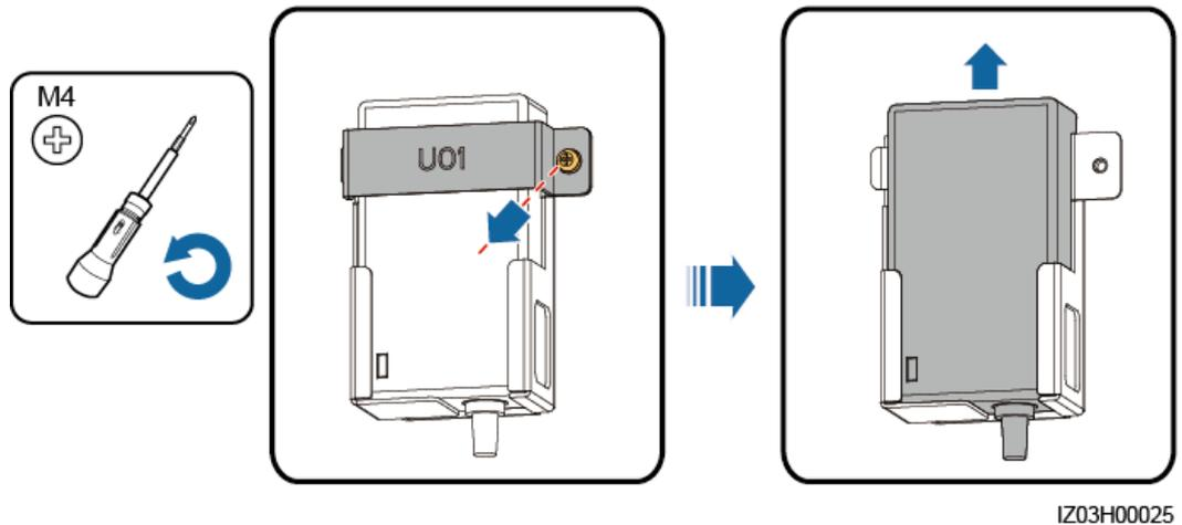
**Step 3** Install a new power adapter.
