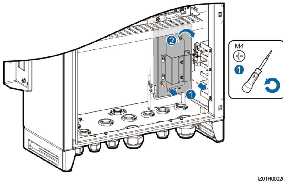
**Step 2** Remove the optical cable fastener.
