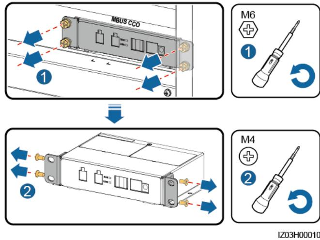
**Step 3** Install the mounting ears on a new SmartMBUS CCO module.
