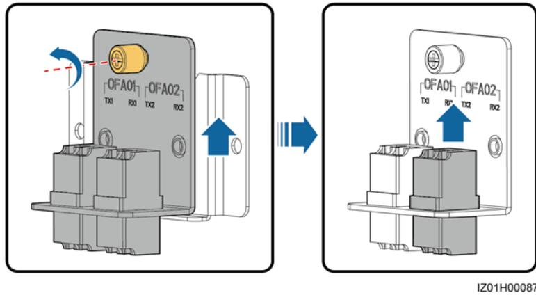
**Step 3** Install a new fiber adapter.
