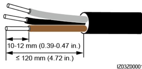
**Step 2** Connect the L1, L2, and L3 wires to the three-phase input switch.
