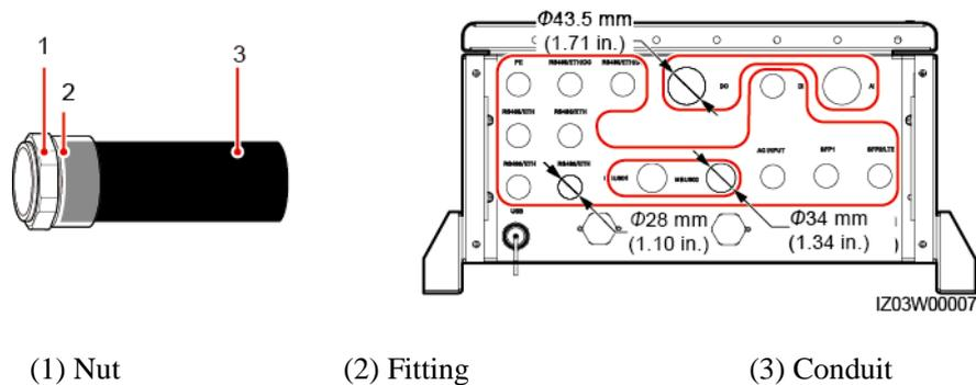
**Step 1** Remove the locking cap and plug from the waterproof connector, and remove the waterproof connector.
