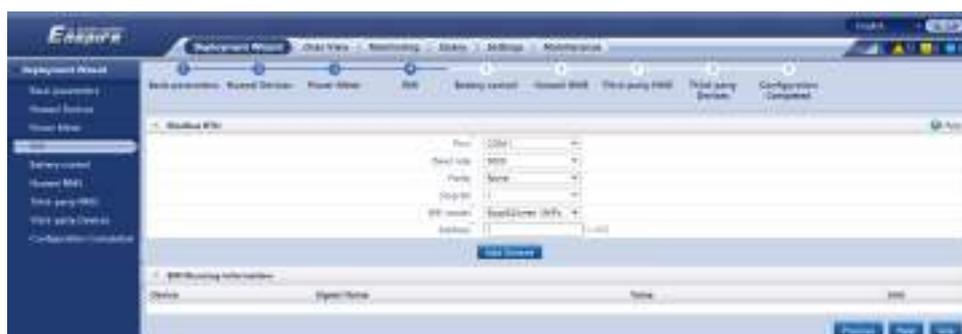
5. Set the battery working mode for battery control.
