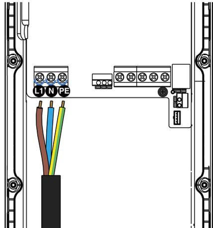
6. Tighten the screws to 2 N·m and fix the cable gland.
