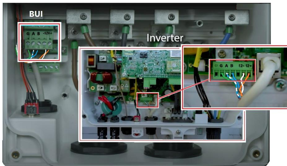
*Figure 5 Communication cable between the BUI and Inverter*
