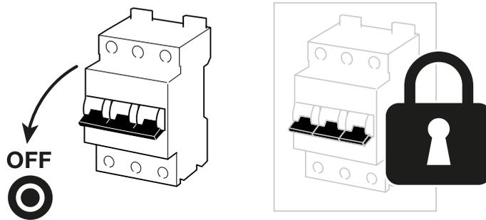
2. Switch DC switch on inverter to **OFF** and secure it against being switched on again.
