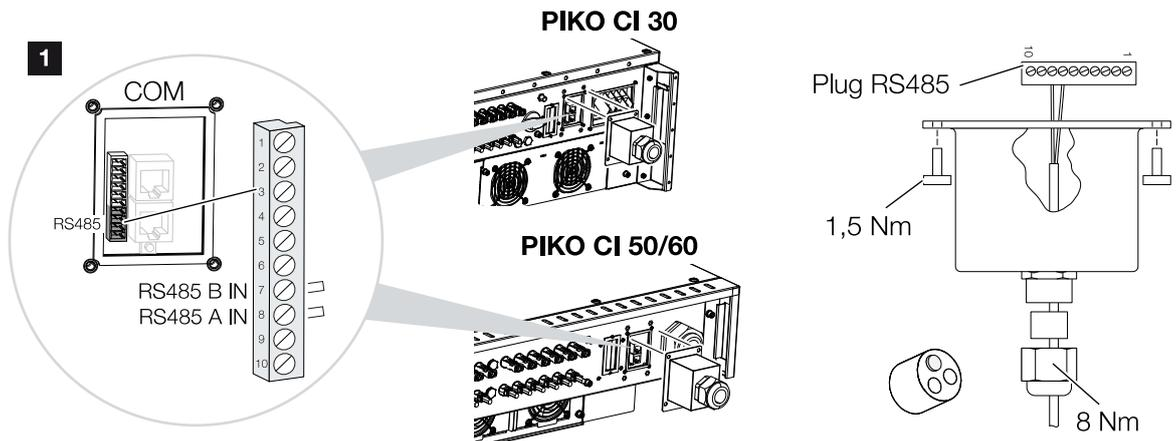
5. Connect the communication cable to the plug connector for the communication interface. Note the pin assignment.
