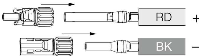
5. Tighten nut on plug connector (3 Nm).
