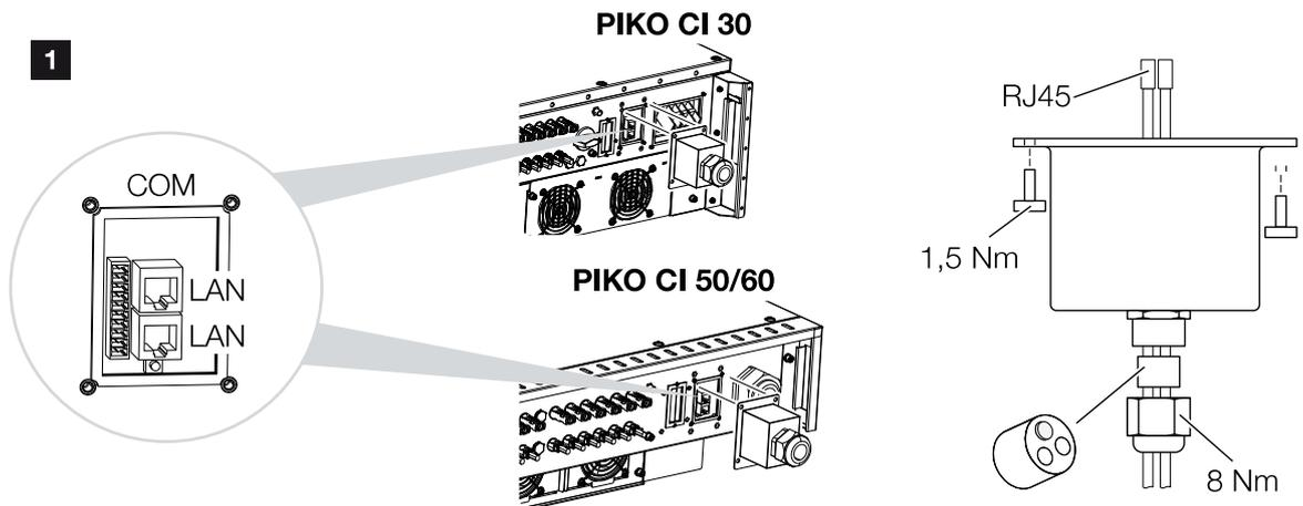
4. Connect Ethernet cable to one of the LAN sockets in the COM2 connection panel. The second LAN socket is used to continue the network connection to further inverters.
