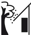
Protect the inverter from coarse soiling, e.g. leaves.
