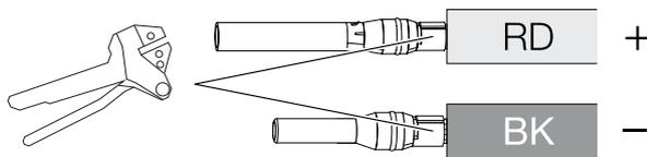
4. Insert contact into plug connector until the contact clicks into place tangibly and audibly.
