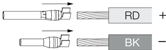
3. Crimp the contact with a suitable crimping tool.
