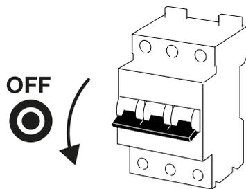
2. Switch the DC switch on the inverter to **OFF**.
