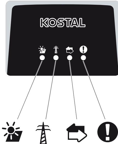
The LEDs on the front indicate the current operational status.
