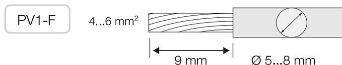
2. Insert stripped wire end into crimped neck of contact.
