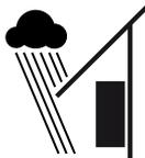
Protect the inverter from direct precipitation.
