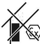
Do not install the inverter in potentially explosive areas.
