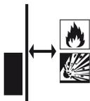
Do not install the inverter on a flammable installation surface.
