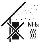
Protect the inverter against dust, contamination and ammonia gases. Rooms and areas containing livestock are not permitted as installation sites.
