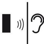
The inverter makes noise during operation. Install inverter in such a way that people are not disturbed by operation noises.
