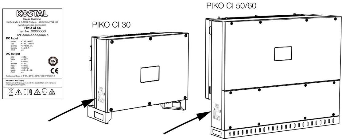
The type plate and other labels are attached to the inverter housing. These signs and labels may not be altered or removed.
