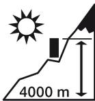
Inverter may only be installed up to an altitude of 4000 m.
