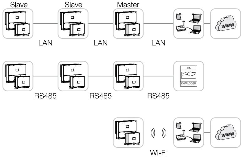
The PIKO CI inverter has interfaces for LAN, RS485 Modbus and WiFi. There are therefore various possibilities for networking one or more inverters with each other and controlling them.
