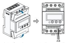
**Step 4** Strip the insulation from the power wires by 10 mm. Then connect the wires
