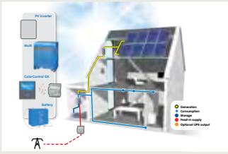
VE Storage Hub-4 is a grid-parallel energy storage system, using the Multi or Quattro bidirectional inverter/charger as its main component.
