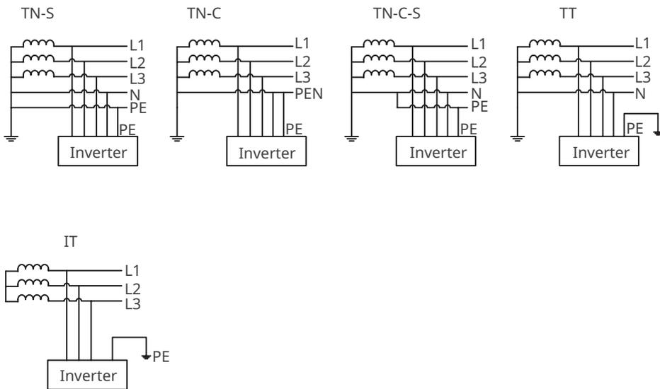
The grid structures supported by GW136K-HTH is IT, as shown in the diagram below:
