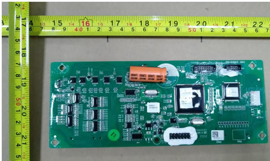
Figure 13. Control board component side view
