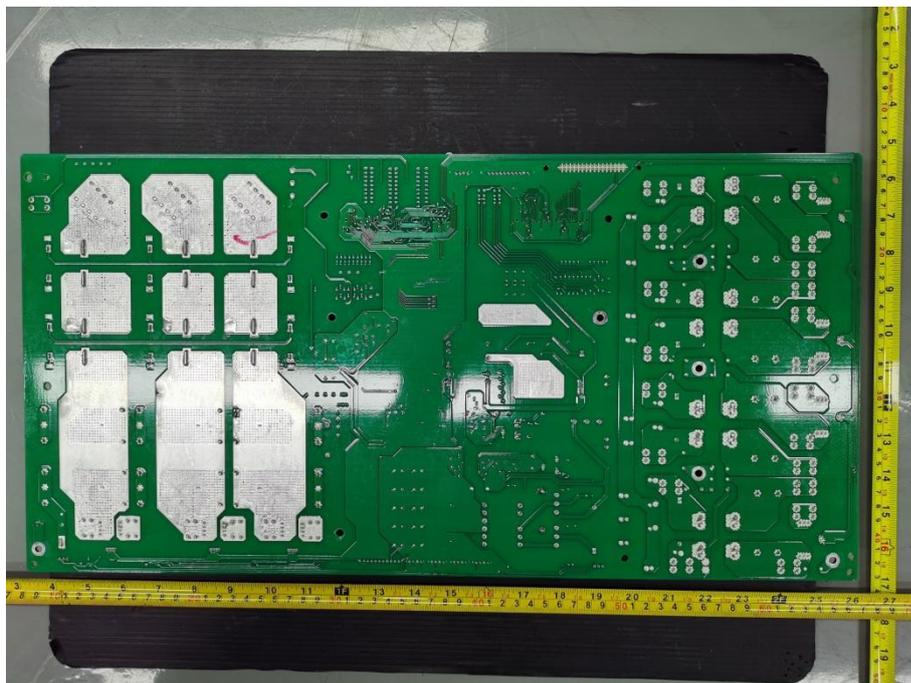
Figure 16. AC board solder side view
