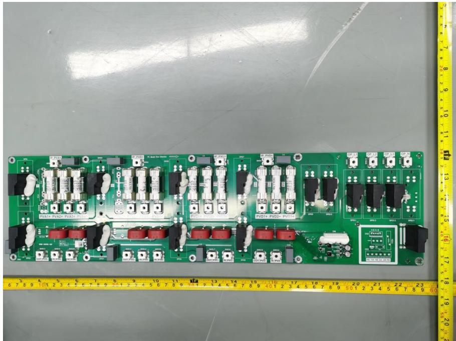
Figure 7. Input board component side view
