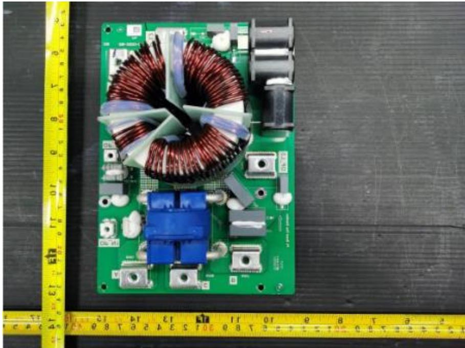
Figure 19. Output board component side view
