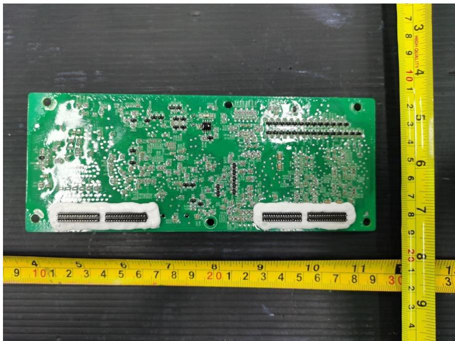
Figure 14. Control board solder side view
