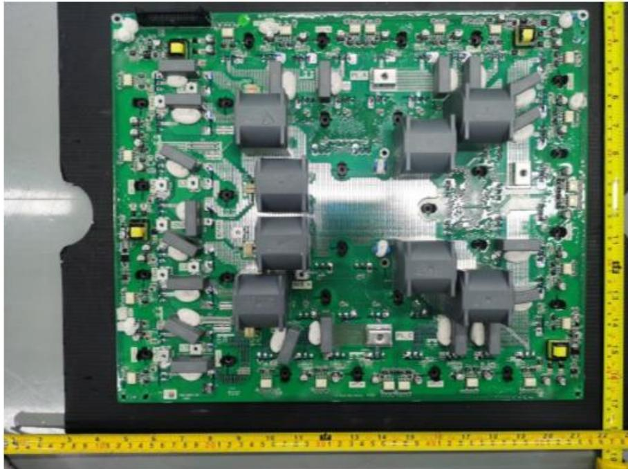
Figure 21. Inverter board component side view
