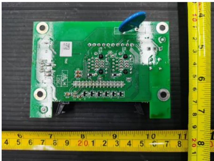
Figure 12. Communication board solder side view
