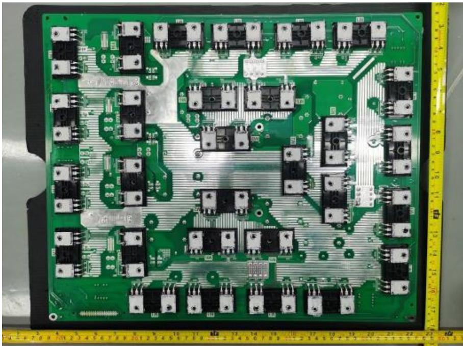
Figure 22. Inverter board component solder view
