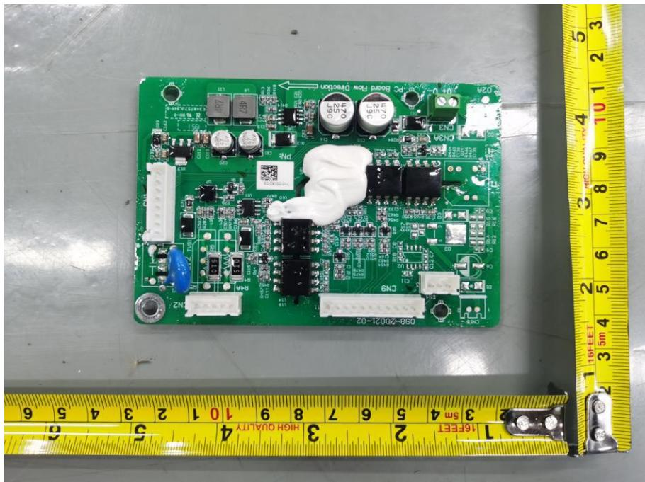
Figure 9. Communication board component side view
