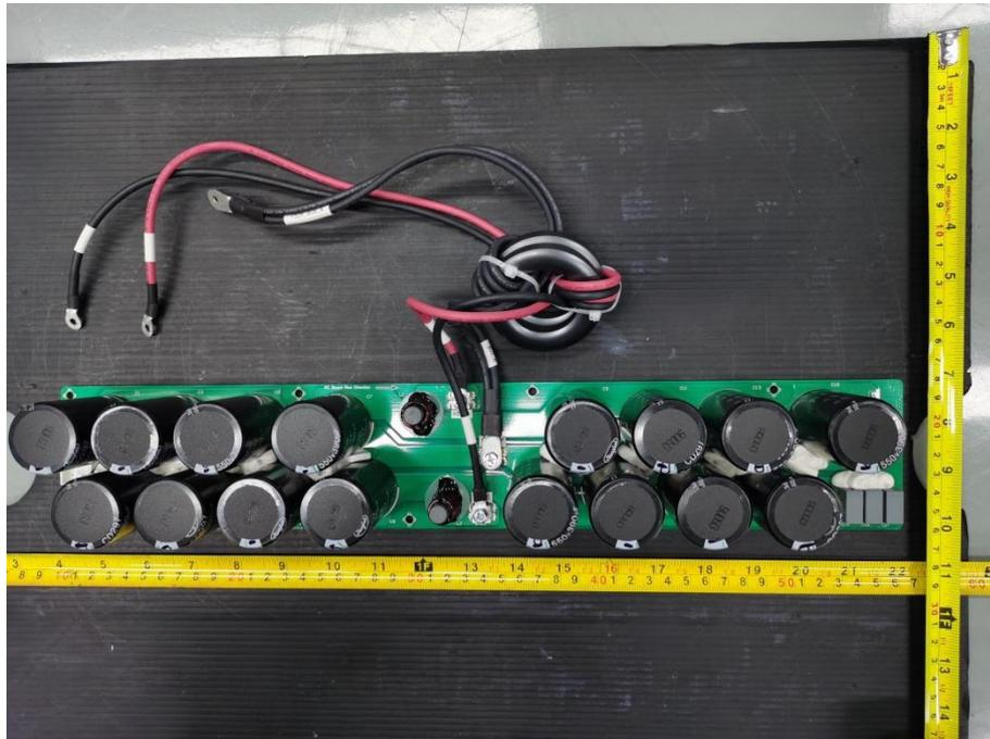
Figure 17. Capacitor board component side view
