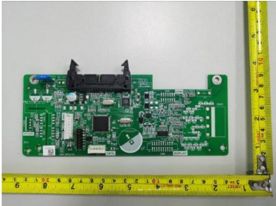
Figure 23.CSB board component side view
