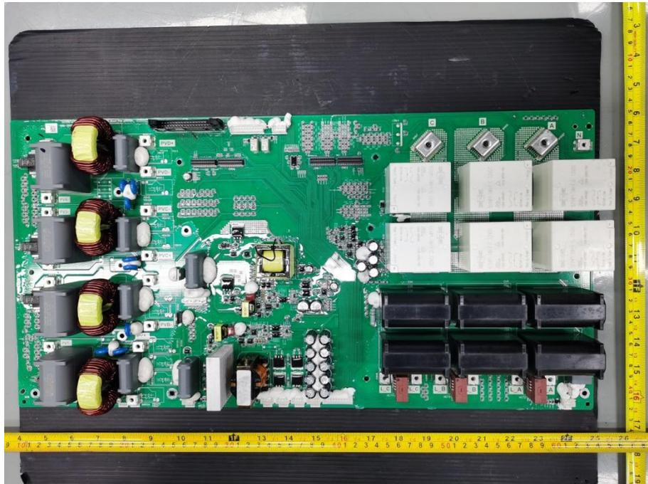
Figure 15. AC board component side view
