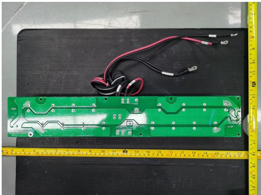
Figure 18. Capacitor board solder side view
