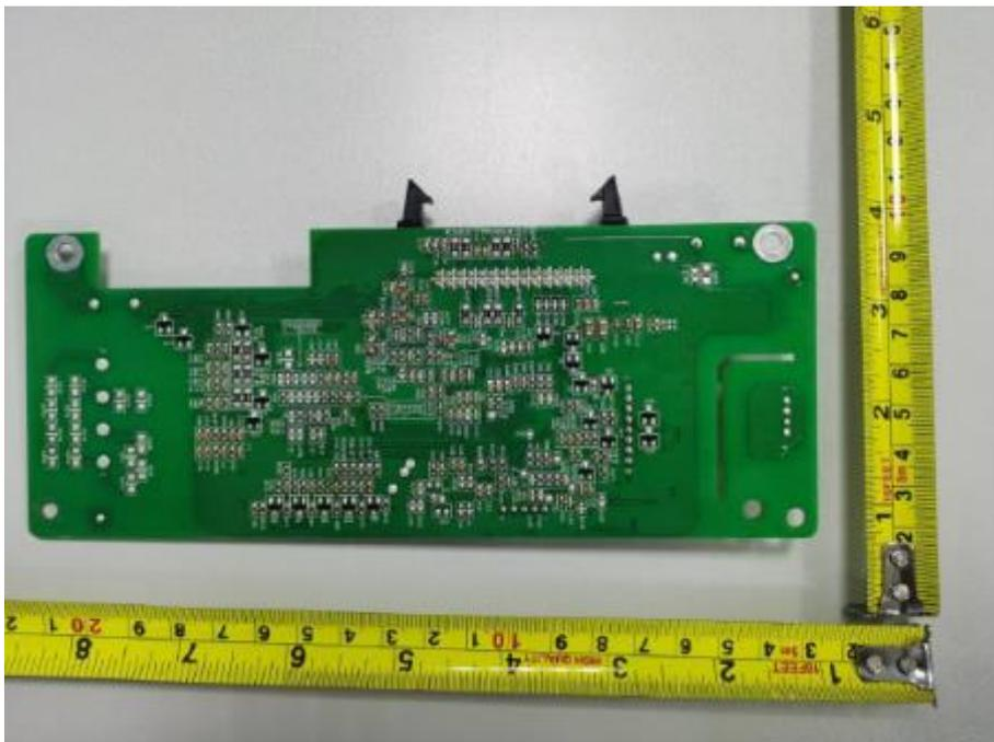
Figure 24.CSB board solder side view
