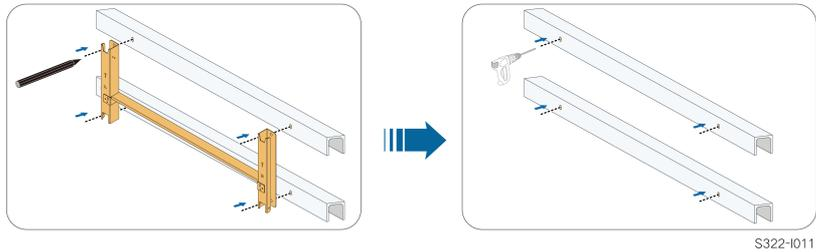
**step 3** Secure the mounting-bracket with bolts.
