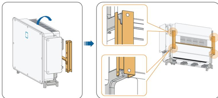
**step 3** Fix the inverter with screws.
