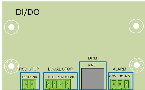
**DO terminal (fault output dry contact)**
