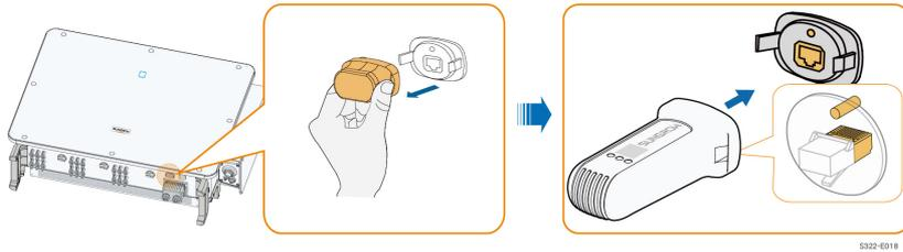
**step 3** Refer to the guide delivered with the module for the set-up.
