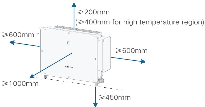
\* In case this distance is less than the distance in the diagram, move the inverter from the mounting-bracket or wall before maintaining fans.
