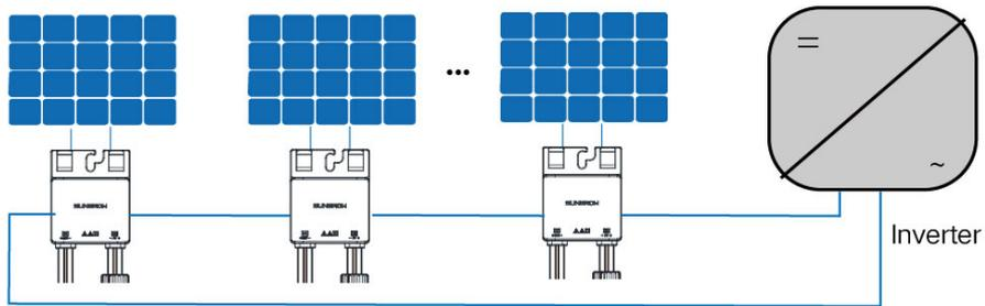
figure 4-2 Optimizers Configured for All PV Modules
